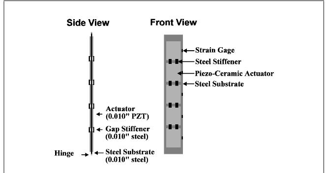
**Figure 3: Front and side views of the composite steel/piezo-ceramic column.** The column is 12.6 inches in length. Steel stiffeners are used to increase the stiffness of the area between adjacent actuators that is not covered by piezo-ceramic material.
