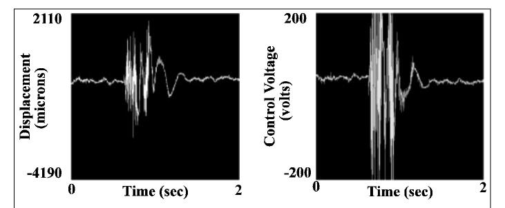
**Figure 5: Response to perturbation.** The plot on the left shows the 1st-mode deflection of the midpoint of the column vs. time. The plot on the right shows the control voltage applied to the center actuator vs. time. The perturbation was induced by banging my fist on the table as hard as I could.
