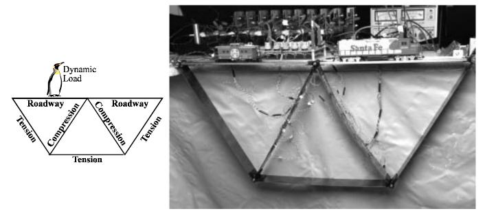
**Figure 7: Actively stabilized truss bridge.** This bridge incorporates two compressive members that actively resist buckling.
