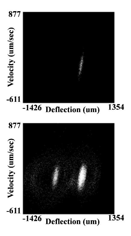
**Figure 6: Phase plots of the system in operation.** The top plot shows the velocity vs. position of the system during normal operation. The bottom plot shows the velocity vs. position of the system undergoing oscillations. This view was created by artificially adjusting the control law so as to induce oscillations that would depict the structure of phase space.
