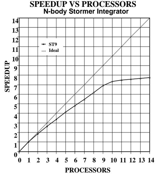
Figure 5: Speedup graph of Stormer integrations. Ample speedups are available to keep the 8-processor *Supercomputer Toolkit* busy, However, the incremental improvement of using more than 10 processors is relatively small.
