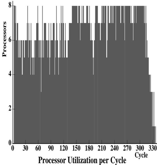
Figure 4: The result of scheduling the 9-body problem onto 8 *Supercomputer Toolkit* processors. Comparison with with the region-level parallelism profile (figure 3) illustrates how the scheduler spread the course-grain parallelism across the processors. A total of 340 cycles are required to complete the computation. On average, 6.5 of the 8 processors are utilized during each cycle.
